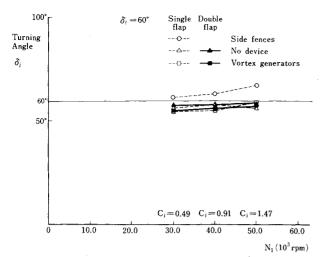
Fig. 5 Effect of side fences on the jet turning performance.
