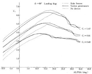
Fig. 7 Effect of side fences on lift characteristics ( $\delta_f$  = 60 deg,  $\beta_u$  = 19 deg).
