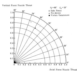
Fig. 6 Thrust vectoring performance.
