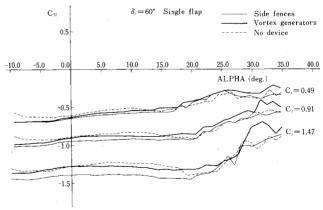
Fig. 9 Effect of side fences on pitching moment coefficient ( $\delta_f = 60$  deg,  $\beta_u = 19$  deg).
