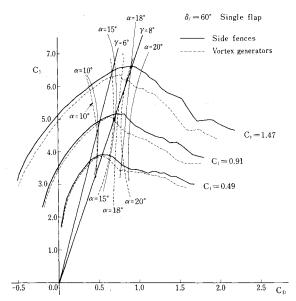
Fig. 10 Lift-drag polars for the landing flap configuration.
